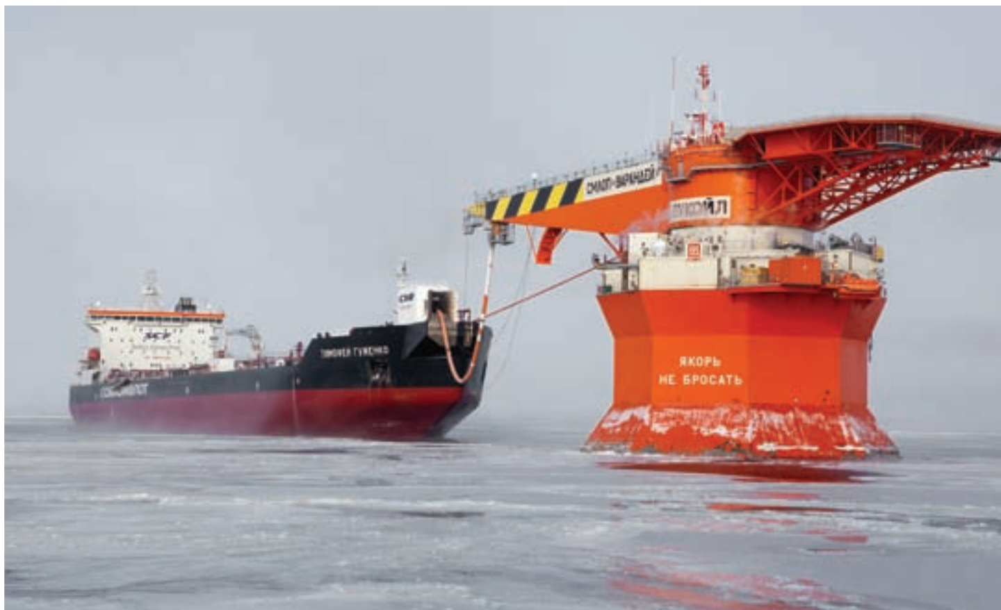
Timofey Guzhenko , 70,000 tonnes dwt Arctic shuttle tanker, at the Fixed Offshore Ice-resistant Off-loading Terminal (FOIROT) at Varandey, Barents Sea, January 2010
